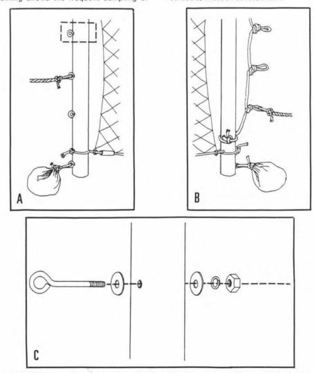
Figure 1. Diagrammatic representation of brail modifications for seine towing. A) Brail with eye bolts. B) Brail with knotted rope replacing eye bolts. C) Exploded view of eye bolt attachment. See text for details.
